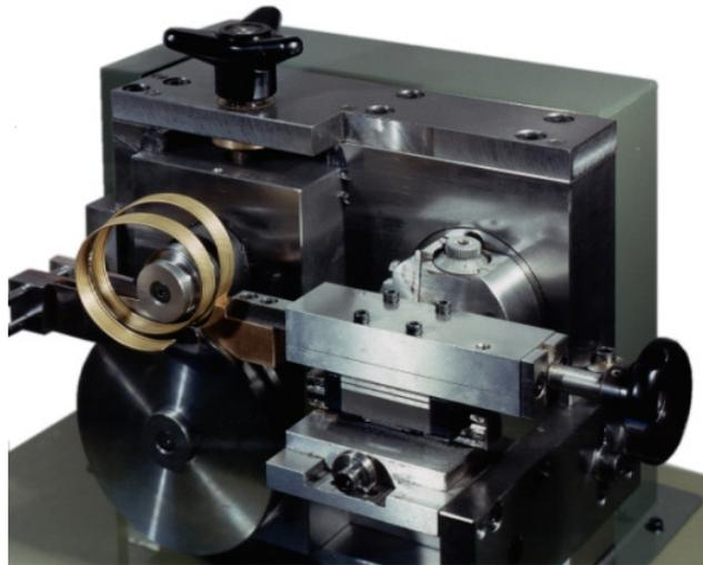
Machine realized to obtain ear-rings and bracelets from plate, by special equipment. The machine is formed by a pair of shaped wheels both motorized. The superior wheel has the possibility to move near and far from the inferior one for obtaining the perfect drag of the plate to be wound in round and oval. The machine is provided also by a particular device that allow an easy adjusting for obtaining round and oval spirals (more or less oval) in different diameter.
