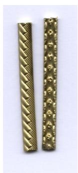
Machine studied and realised for shaping wires and tubes by means of grooved small wheels. In accordance with the small wheels, we can obtain, starting from round wires, flat wires, half-round wires, oval wires, etc.
