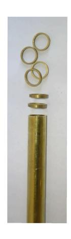
The saw machine for cutting the tube is designed to realize blanks for the realization of wedding rings without any soldering starting from tube.
