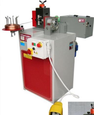
Machine studied and realized for shaping wires and tubes by the use of grooved small wheels. In accordance with the small wheels, we can obtain, starting from round wires, flat wires, half-round wires, oval wires, etc.
